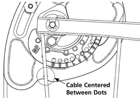
Figure 3: Cam Timing
