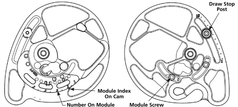
Figure 2: Conventional Binary Draw Length Adjustment
