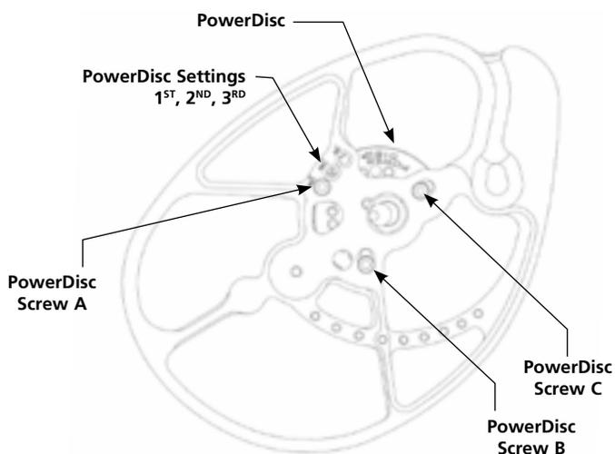
Figure 3: PowerDisc Adjustment
