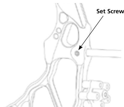
Figure 5: Adjusting the string stop
