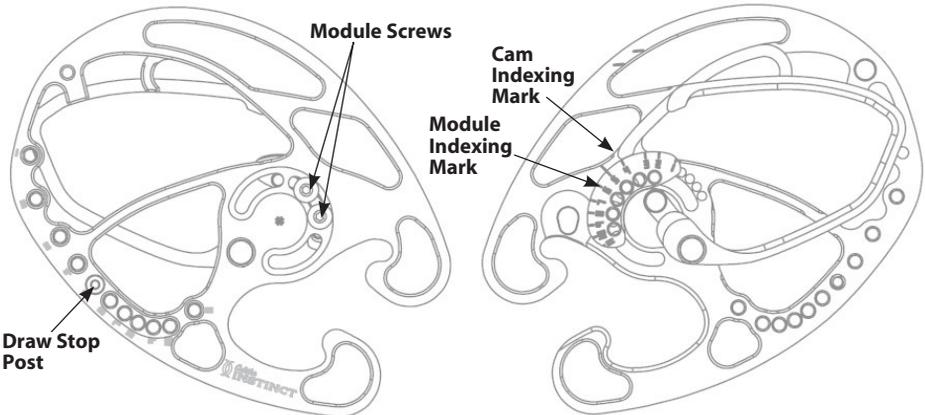
**Figure 1: Xcite Cam System draw length adjustment**
