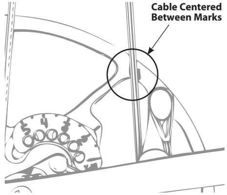
**Figure 2: Xcite Cam System Timing**
