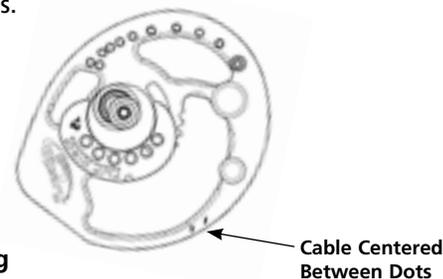
Figure 6: Cam Timing
