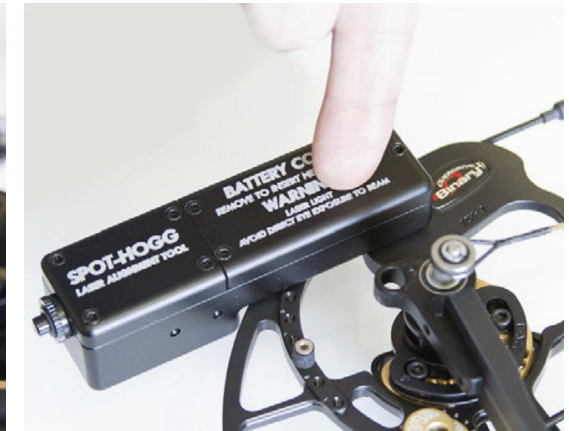
Fig. 3 - DO hang the larger portion of the laser tool off the edge of the cam.
