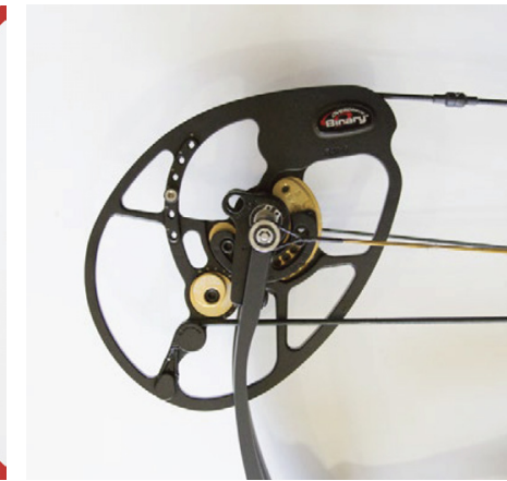
Fig. 1 - Use the power side (side with the module) for laser adjustments.
