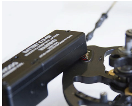
Fig. 2 - DO NOT sit the laser tool on any raised area of the cam.
