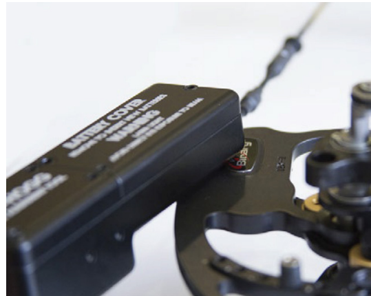
Fig. 2 - DO NOT sit the laser tool on any raised area of the cam.
