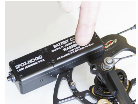
Fig. 3 - DO hang the larger portion of the laser tool off the edge of the cam.
