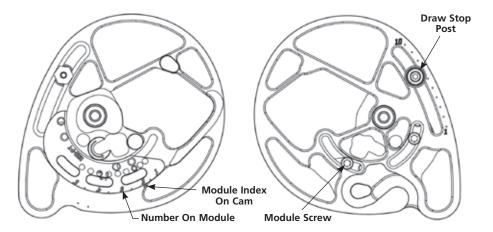
Figure 2: Conventional Binary Draw Length Adjustment
