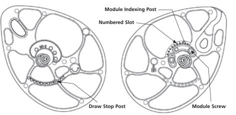
Figure 1: OverDrive Binary Draw Length Adjustment
