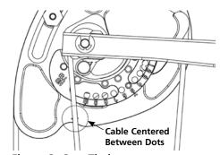
Figure 3: Cam Timing
