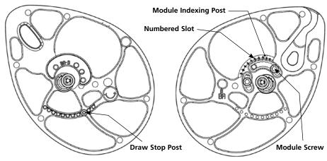
Figure 1: OverDrive Binary Draw Length Adjustment
