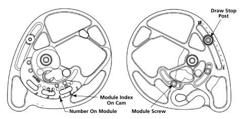
Figure 2: Conventional Binary Draw Length Adjustment
