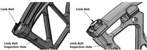
Figure 5: Draw Weight Adjustment (Insanity CPX, Insanity CPXL, Invasion CPX, Assassin, Assassin SD and HeartBreaker)
