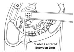
Figure 3: Cam Timing
