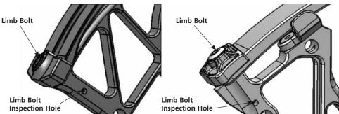
Figure 5: Draw Weight Adjustment (Experience, Insanity CPX, Insanity CPXL, Assassin and HeartBreaker)
