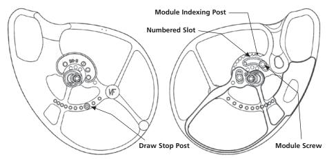
Figure 1: OverDrive Binary Draw Length Adjustment
