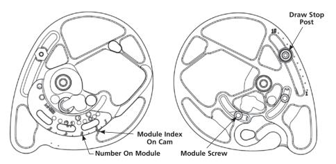
Figure 2: Conventional Binary Draw Length Adjustment
