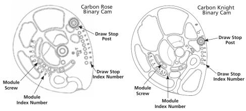
Figure 2: Conventional Binary Draw Length Adjustment
