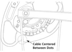
Figure 3: Cam Timing
