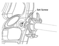
Figure 6: Adjusting the string stop
