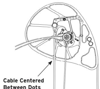
**Figure 8: Cam Timing**
