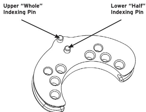
Figure 1: Realm SR6 FlipDisc Mod with dual pins
