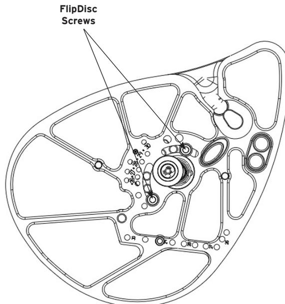
**Figure 4: FlipDisc Adjustment**
