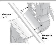
Center shot can be set by measuring from the back of the riser to the arrow and then from the front of the riser to the arrow. Once this is equal, you are at the approximate center shot of your bow (see
